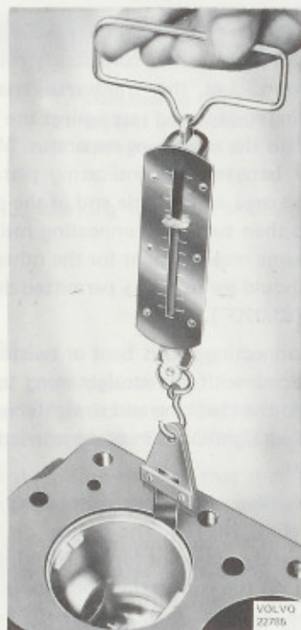
Fig. 21-27. Measuring the piston clearance
